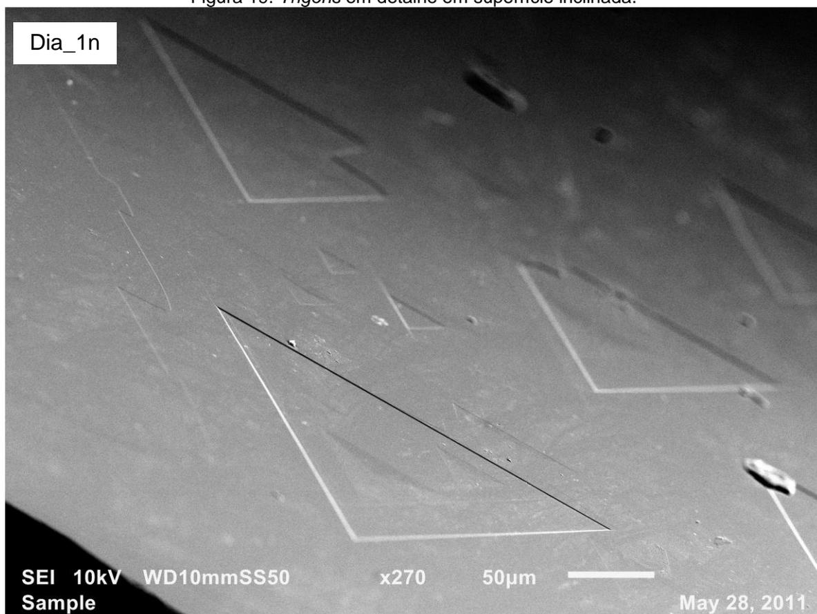
Figura 20: Presença de *tetragons* observada em superfície cúbica.
